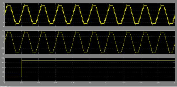
Fig. 10. Simulated Output of HERIC Topology
