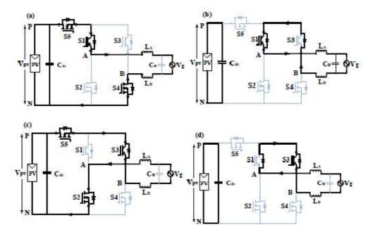
Fig.1. Operation modes of H5 topology. (a) Active mode in the positive half period. (b) Freewheeling mode in the positive half period. (c) Active mode in the negative half period.(d) Freewheeling mode in the negative half period.
