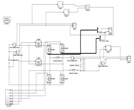
Fig. 8 Simulation of H6 Topology
