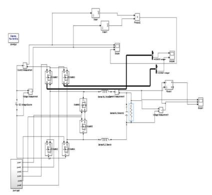
Fig. 7. Simulation of HERIC Topology
