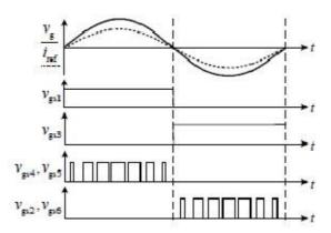
Fig. 4. Schematic of gate drive signals with unity power factor
